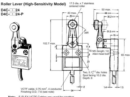
Note: S-FLEX VCTF Cables are used for weatherresistant models (D4C-P).
